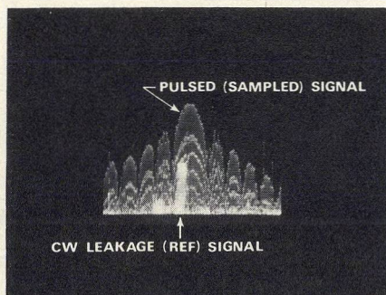
7. IF gating method allows a small level of CW leakage that can be used as a reference.
